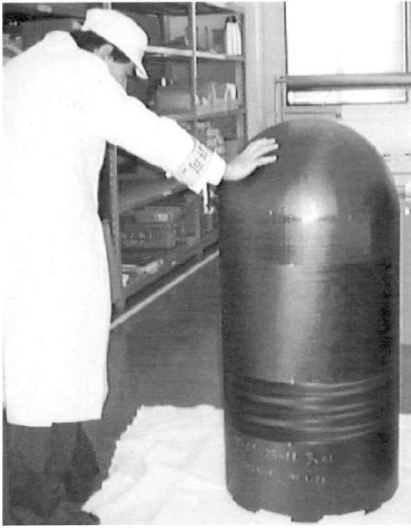
Figure 8. 60 cm lay-up and cryogenic test configuration.
