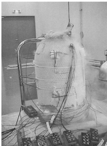
Figure 6. Cryogenic testing of the small FW tank.
