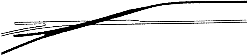
Figure 3. Deformation of the Y-joint.
